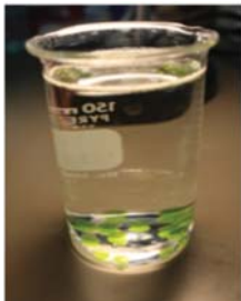
Fig. 5 - Sinking leaf disks in bicarbonate solution.
